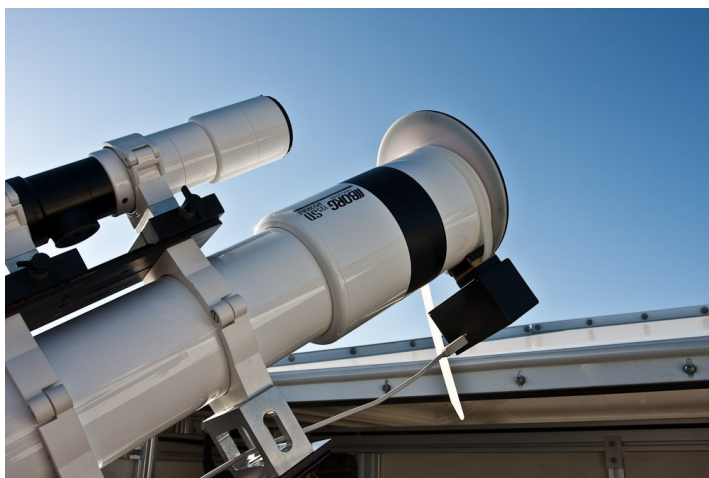
Figure 3 (left): Flip-Flat installed on Borg 125SD in closed position; Figure 4: Flip-Flat in open position, ready to image.
