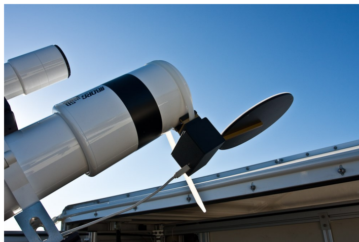
Figure 3 (left): Flip-Flat installed on Borg 125SD in closed position; Figure 4: Flip-Flat in open position, ready to image.
